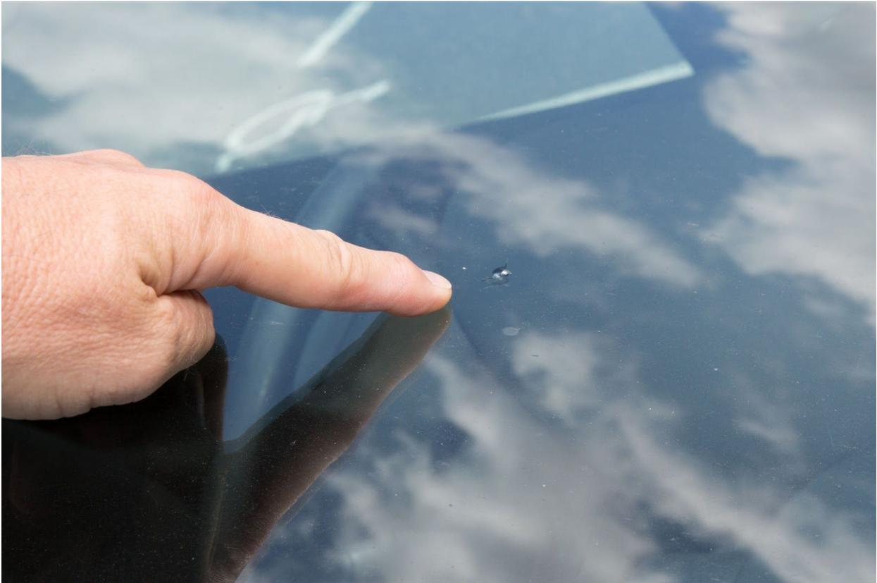
Rock chips on your windshield aren't just an eyesore, they play an important role in your safety. Damaged windshields are best addressed immediately after the damage occurs. Whether or not the chip can be easily fixed, or the windshield needs a complete replacement, depends on a few different factors.
